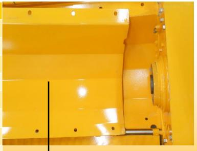
Replaceable Wear Sheet Being Installed
